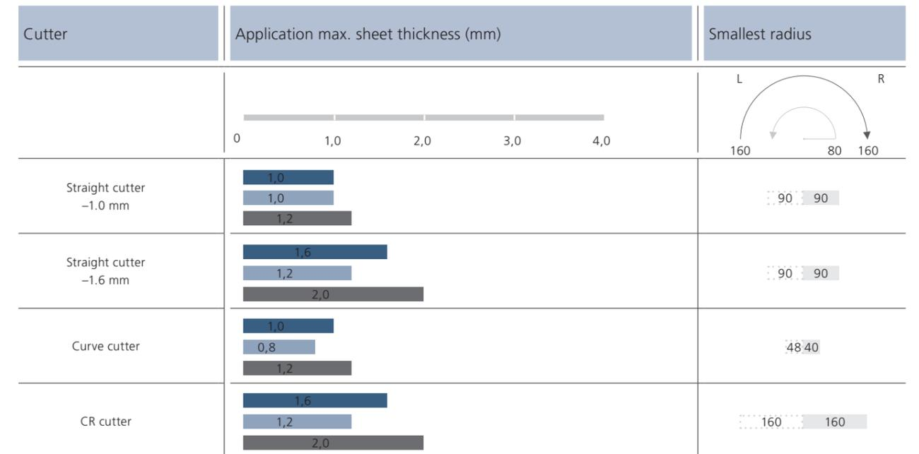
■ Steel (400 N/mm<sup>2</sup>) ■ Stainless steel (600 N/mm<sup>2</sup>) ■ Aluminium (250 N/mm<sup>2</sup>)
