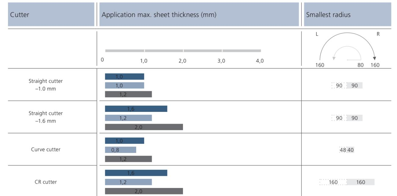
■ Steel (400 N/mm<sup>2</sup>) ■ Stainless steel (600 N/mm<sup>2</sup>) ■ Alu (250 N/mm<sup>2</sup>) ■ Spiral ducts
