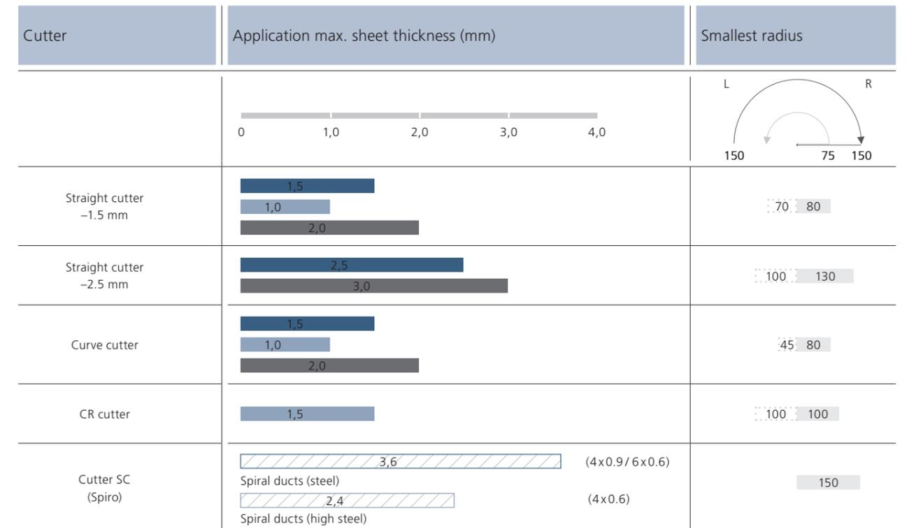
■ Steel (400 N/mm<sup>2</sup>) ■ High steel (600 N/mm<sup>2</sup>) ■ Aluminium (250 N/mm<sup>2</sup>) ■ Spiral ducts
