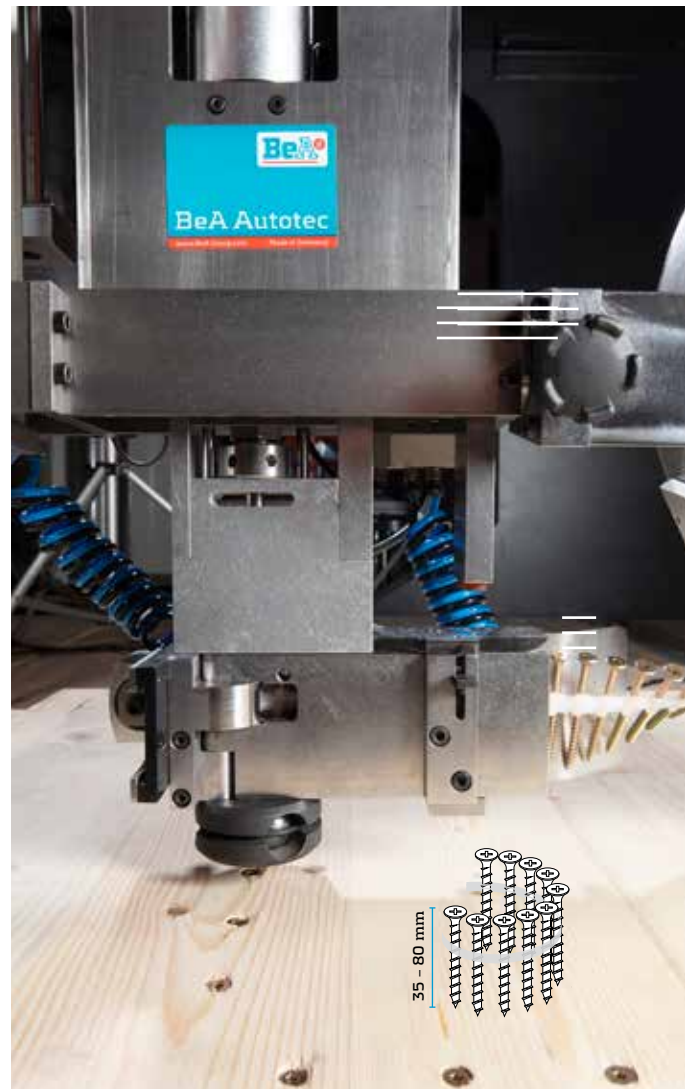
Jumbo coil: Magazine capacity 700 Screws
